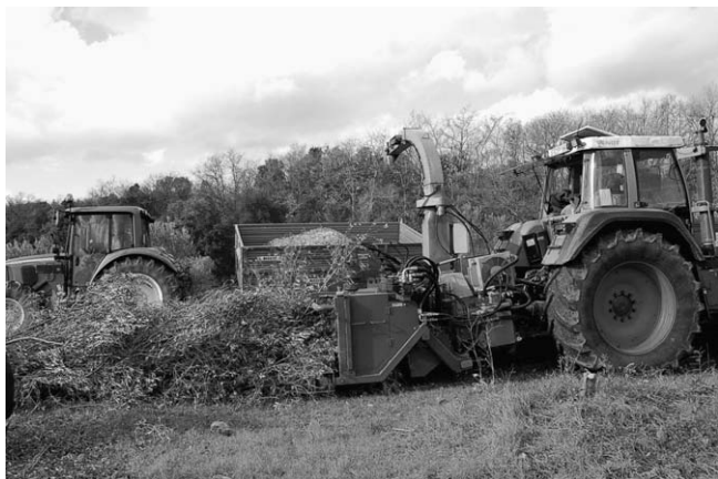
Fig. 1. Tractor-mounted machine while harvesting olive pruning residues. The high-tipping bin is not installed here and biomass is blown onto a towed trailer.
