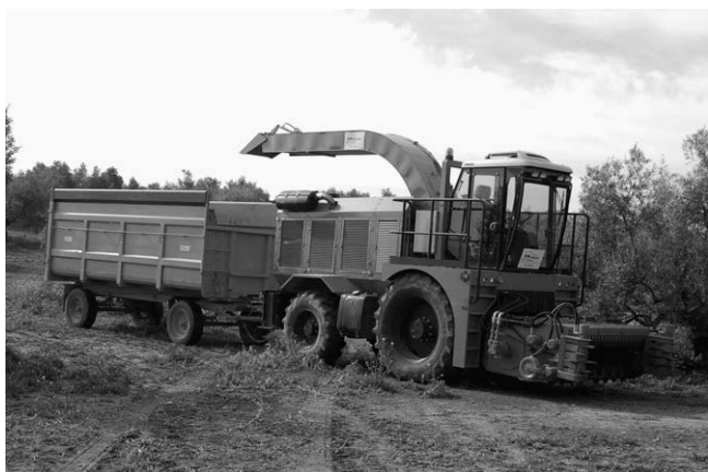
Fig. 2. Self-propelled machine complete of 22 m 3 bin trailer.
